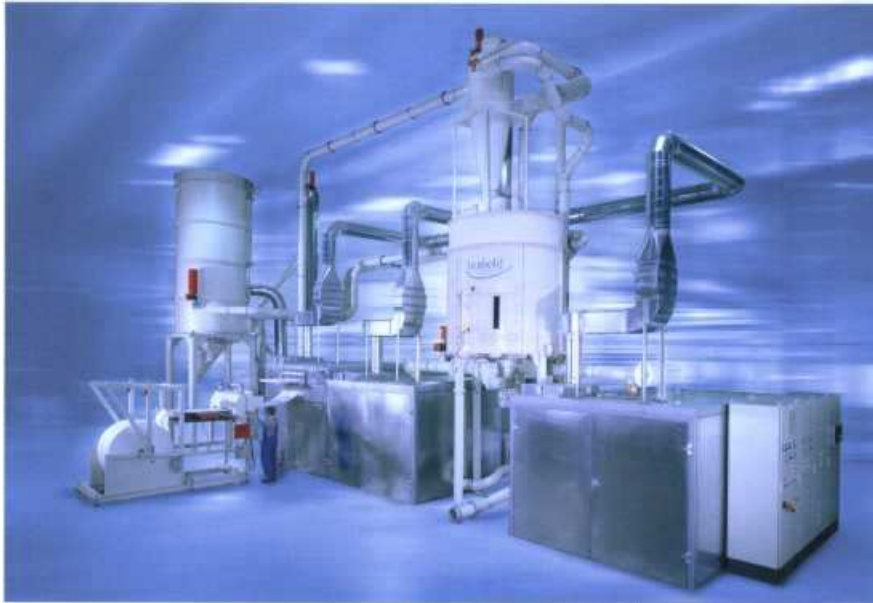
Complete line for the pulverization of cellulose with explosion proof protection
